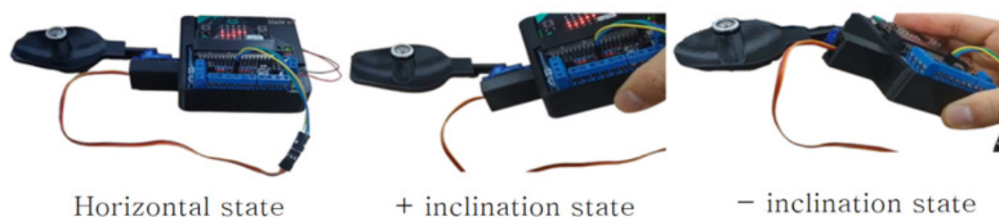
Fig. 7. Tilt-compensation test on the x-axis of the ‘Tilt-Compensation Spoon’ model
